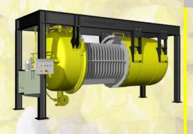
With the choice of the Liquid Sulphur Filter system the sulphur quality is established. Straining is coarse filtration for the protection of the sulphur burners or the openings in sulphur forming equipment. Liquid Sulphur Pre-coat Filters and Polishing Filter are used for the protection of the catalyst bed in sulphuric acid production. Based on the requirements we size and produce Liquid Sulphur Filters.
